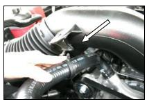
1. **Disconnect the negative battery cable!** Lift up on the front of the and beauty cover and remove it from the vehicle. Push down on the radiator hose, and separate the tube from the plastic clamp.
