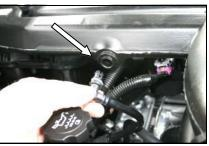
**2.** Disconnect the breather tube from the intake tube, by gently pulling towards you. An O-ring is all that holds it in place. Next loosen the hose clamp on the intake tube at the throttle body, and at the Mass Air Sensor, and remove the tube from the vehicle.
